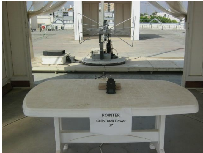
Figure 3. Radiated Emission Test
