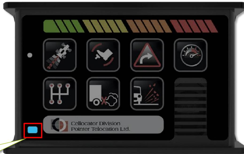
Status LED blinking continuously.
