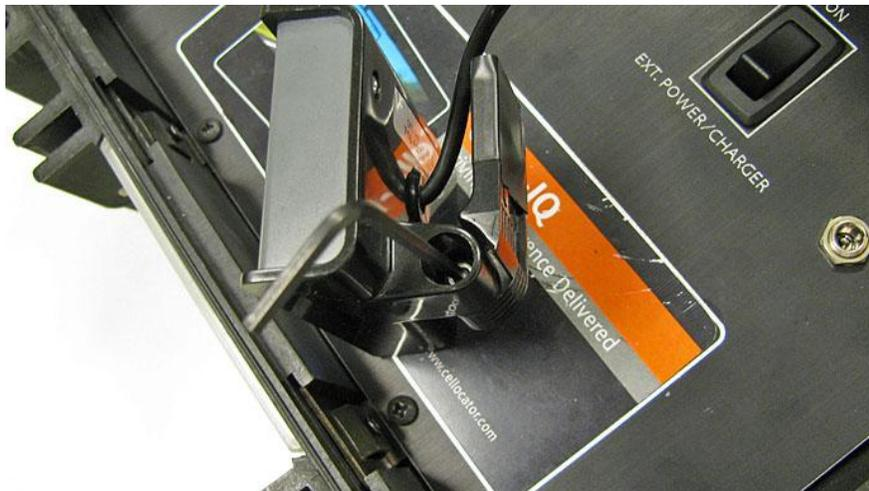
Figure 9: Adjusting the angle of the DFD fitting stand
