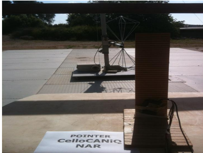
Figure 3. Radiated Emission Test
