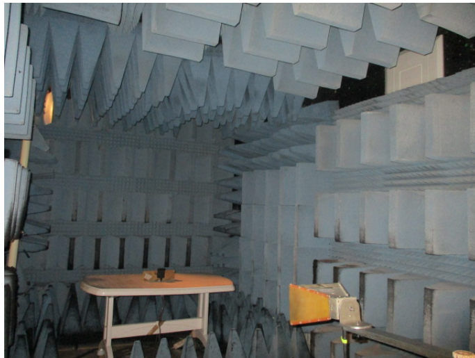
Figure 5. Immunity to Radiated Field Test Above 1 GHz
