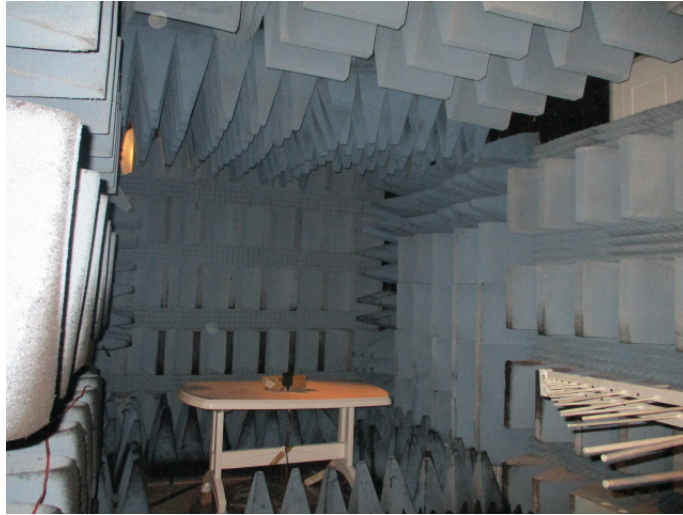
Figure 4. Immunity to Radiated Field Test Below 1 GHz
