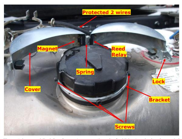
The stainless steel Fuel Cap Sensor is mounted on the fuel lid using the bracket and three Allen screws. A lock is used to close the two parts of the cover. The spring enables automatic opening of the cover when the lock is opened. When the cover is closed, the reed relay is adjacent to the magnet and the two wires are connected to each other. When the cover is opened the reed relay opens the circuit and disconnects the two wires.
