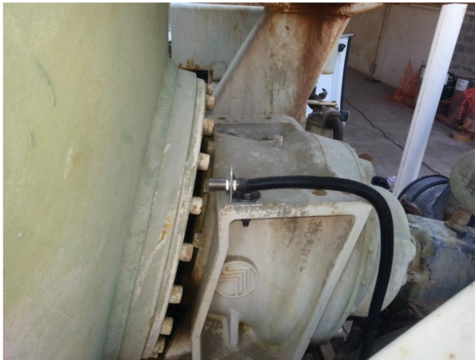
Figure 2: Attaching the Concrete Mixer Sensor
