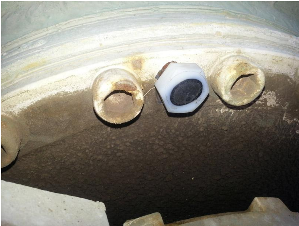
Figure 1: Installing the Concrete Mixer Sensor Bolts
